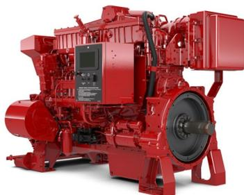
The Cat® 3406C Industrial Diesel Fire Pump Engine is offered in ratings ranging from 218-359 kW (292-482 bhp) @ 1750-2300 rpm. These ratings are non-certified and available for global non-regulated areas. They are FM Approved and UL Listed. Additional 3406C ratings with or without radiators are available, but not FM approved or UL listed. Starting on demand is a must for a fire pump engine - always. Cat® fire pump engines have a reputation for reliable starts and long efficient service.
