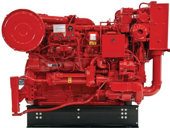
Cat® 3508 Industrial Diesel Fire Pump Engines, with ratings: 709-794 kW (950-1065 bhp) @ 1460-1750 rpm, are non-certified, not FM Approved, and not UL Listed. They are available for global non-regulated areas. Starting on demand is a must for a fire pump engine - always. Cat® fire pump engines have a reputation for reliable starts and long efficient service. The Cat line of fire engine pumps covers a wide range of installations.
